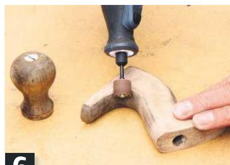
**6** Remove old lacquer from handles with Dremel tool and hand sanding. Bleach wood if surfaces patchy
